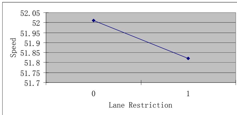
Figure 79 Restrictions to Truck Sensitivity on Running Speed after FA
